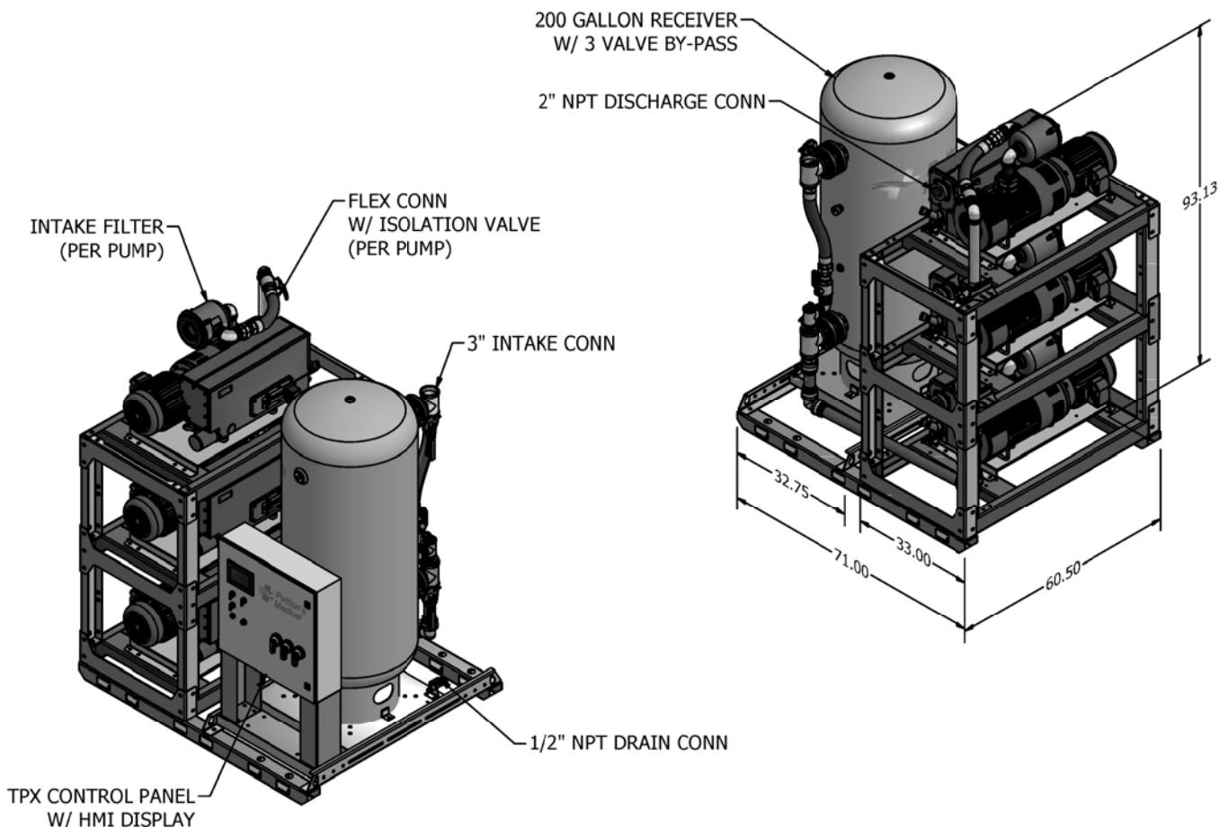
**Triplex Lubricated Rotary Vane Medical Vacuum Package Specifications<sup>1</sup>**
