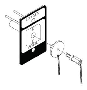
The Locking Kit shall prevent tampering of the internal primary check valve, located in the latch valve assembly.
