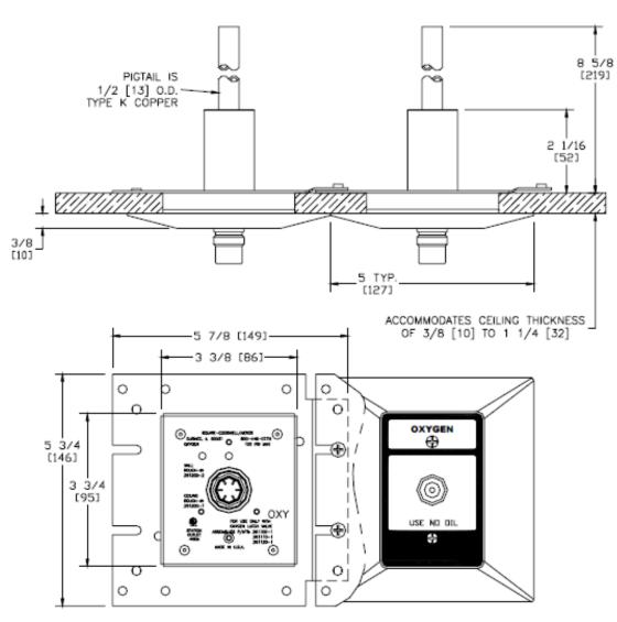
ROUGH-IN ASSEMBLIES TO BE MOUNTED TO COLUMN, PIPING CAN NOT SUPPORT WEIGHT OF OUTLET ASSEMBLY.
