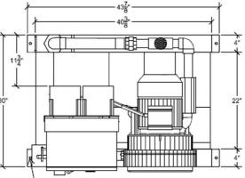
USE (4) 1/2" CONCRETE WEDGE ANCHORES TO MOUNT TO HOUSEKEEPING PAD TO MEET SEISMIC CODE.
