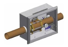
The valve shall be 3 piece ball-type with a full port design. All valves shall be serviceable in the line, supplied clean and prepared for oxygen service. The valve shall have a bronze body and a blow-out proof stem. The valve ball shall be bronze chrome plated and the seats and packing shall be Reinforced Teflon (PTFE). The valve shall also have a continuous pressure of up to 600 psi and vacuum service to 29" Hg.
