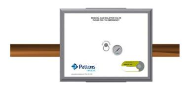
The zone valve box shall be constructed of 18 gauge steel complete with a baked white enamel finish. The box shall be equipped with two adjustable steel brackets for the purpose of mounting the box to the structural support. The steel brackets shall accommodate various finished wall thicknesses between 3/8" [9.5 mm] and 1-3/16" [30 mm] and shall be field adjustable.
