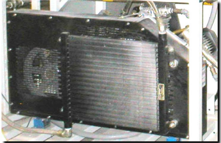
When some companies need to add an aftercooler to their package, they usually slap it on the outside of the belt guard and run some piping to it. This makes changing or adjusting the belts rather difficult. Most times you have to disconnect the piping in order to take off the guard's front cover. This can be awkward, heavy and increase the chance of damage or an air leak after reassembly.
