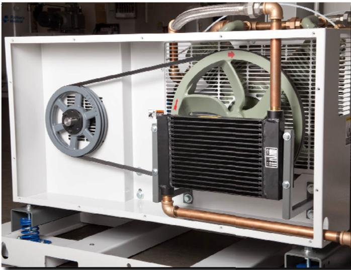
At Patton's Medical, we placed the aftercooler inside the guard allowing for the appropriate distance from the flywheel for proper cooling. The piping does not interfere with the belt guard cover and the belts can therefore be easily removed or adjusted. We also added slotted holes and adjustment screws to the compressor/motor base to help slide the motor for more accurate belt adjustment.
