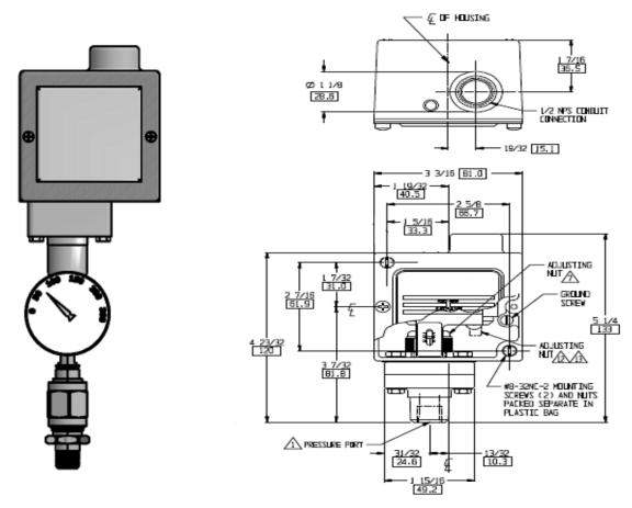
Pressure Switch Gauge Assembly
