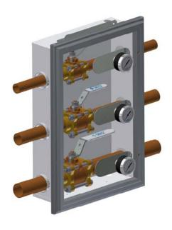
The valve shall be 3 piece ball-type with a full port design. All valves shall be serviceable in the line, supplied clean and prepared for oxygen service. The valve shall have a bronze body and a blow-out proof stem. The valve ball shall be bronze chrome plated and the seats and packing shall be Reinforced Teflon (PTFE). The valve shall also have a continuous pressure of up to 600 psi and vacuum service to 29" Hg.
